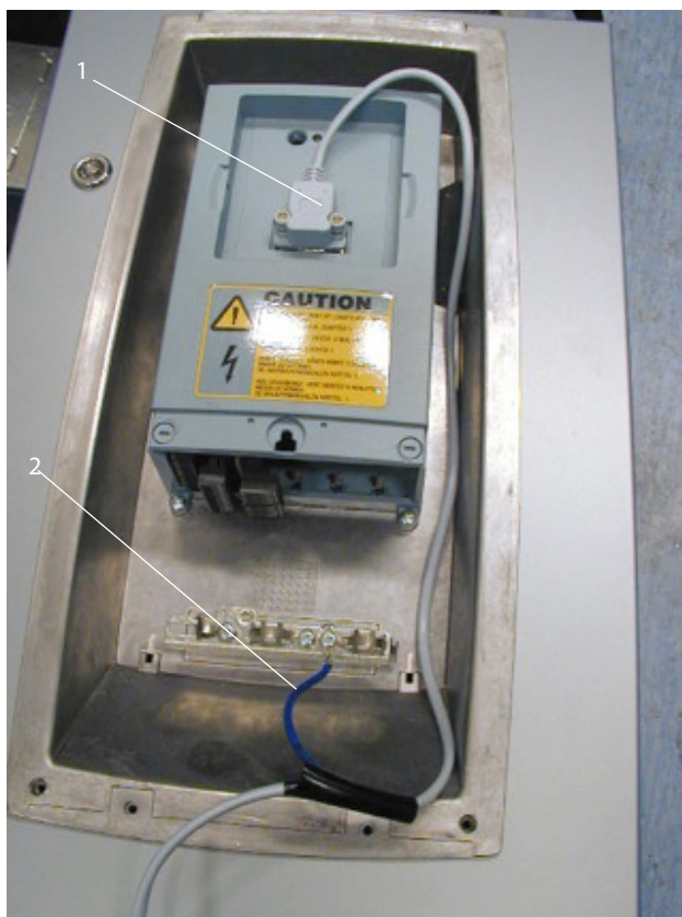
Illustration 3: Connection of VACON cable and the grounding cable, FR8
