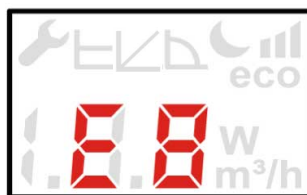
Fig. 16: Display of error code E8 (motor fault)
