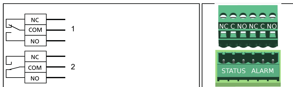
Fig. 10: Wiring diagram for the "in operation" message
