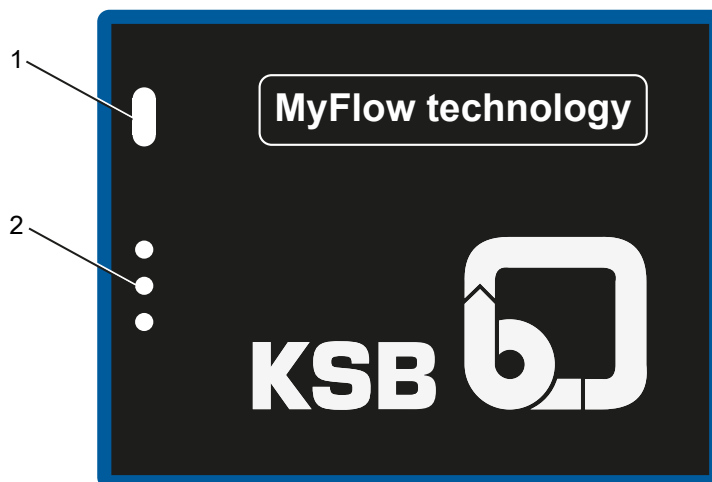
III. 28: Interface Service et LED de signalisation
